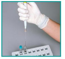
Insert capillaries filled with 10 µl blood, into TRI 142- and CHO 142-cuvettes, respectively
