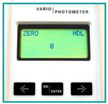
Insert non-treated HDL 321-cuvette into photometer (blank value)
