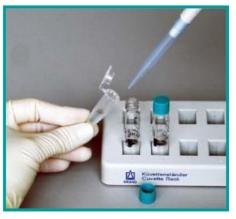
Pipette 500 µl supernatant into HDL 321-cuvette
