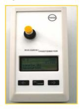
Afterwards insert cuvette in photometer
