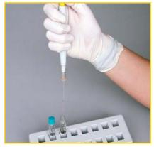
Add sample and wash out the capillary with reagent solution with micropipettor
