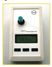
Insert cuvette with biodiesel sample in photometer (blank value); photometer saves blank value
