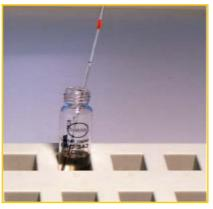
Insert capillary in cuvette
